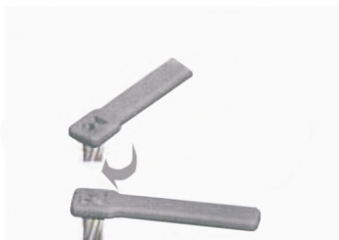
3. A part of wrench and B part of insert must be parallel to each other before clamp the insert. Turn the wrench clockwise to finish clamping.
